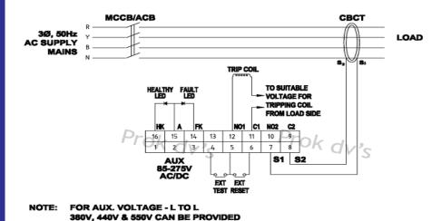
WIRING DIAGRAM FOR DIGITAL MICROCONTROLLER / MICROPROCESSOR BASED EARTH LEAKAGE RELAY(ELR) WITH CORE BALANCE CURRENT TRANSFORMER (CBCT / ZCT)(DMPEL SERIES) - DIN MOUNTING-RS 485 MODEL
