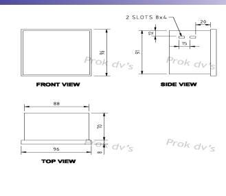
NOTE: ALL DIMENSIONS ARE IN MM TOLERANCE:-±1MM
